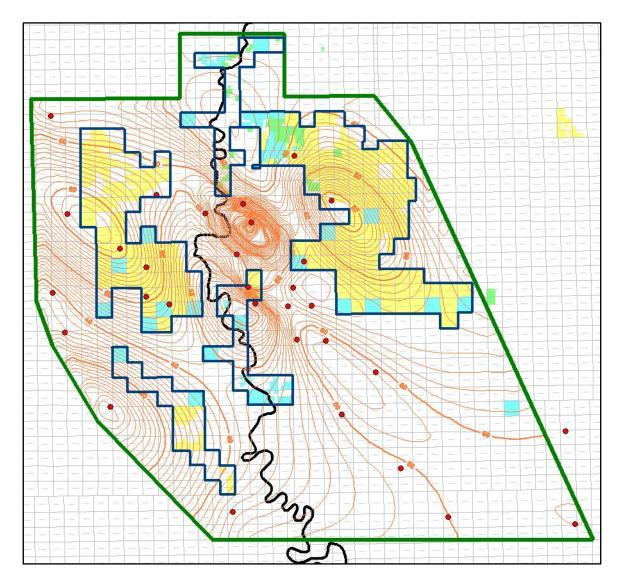
Figure 10: Gross Thickness Isochore of Zone of Interest 5 Showing Evaluation Area Polygon (green), Ryder Scott Prospect Areas (dark blue) and 31 Points of Well Control Utilized.
