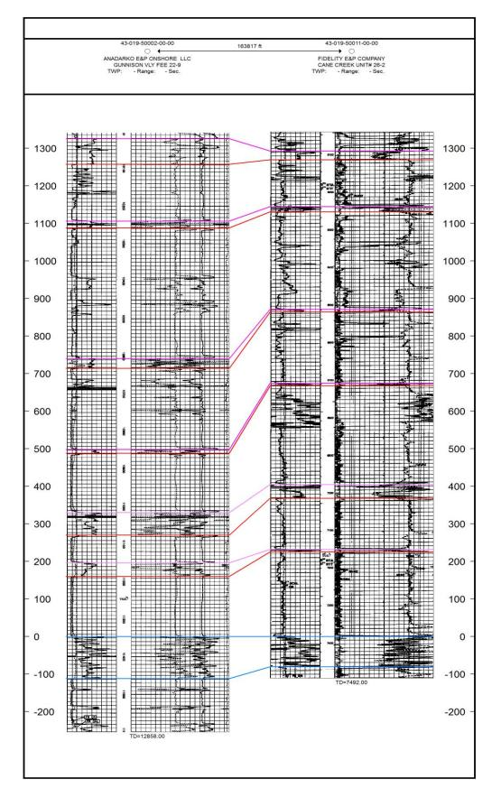
Figure 8: Continuity of ZOI 13-21. Cane Creek producing interval in blue.
