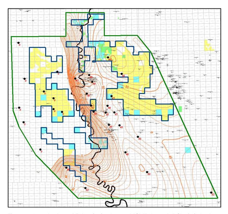
Figure 16: Gross Isochore of ZOI 19 (variously named "C" Marker or "O" Clastic in local correlations).
